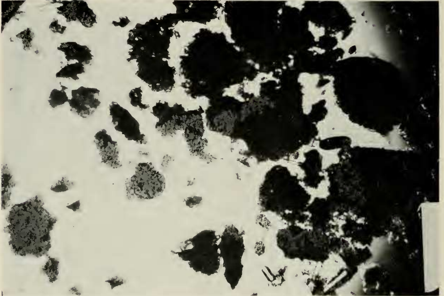
FIGURE 2. Sample fumed with H_2SO_4 , washed and retained on 400-mesh screen.
